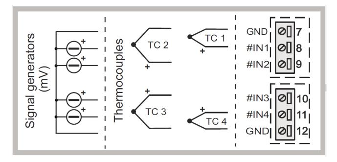
To decrease the signal-acquisition errors due to noise effects, short-circuit each unused TC-type input (screw terminals 8, 9, 10 or 11) to the GND (equipotential screw terminals: 7 or 12).
